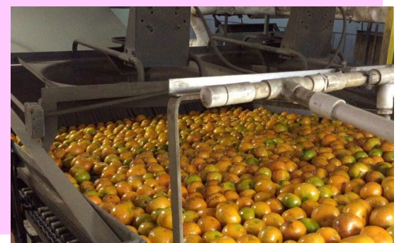
Above: Oranges are conveyed over the packing line for cleaning, sorting, sanitation and packing.
