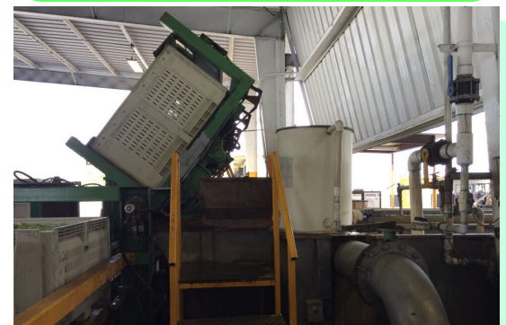
Below: Mechanized tipping systems are used to gently transfer large quantities of produce out of bins and onto packing lines.
